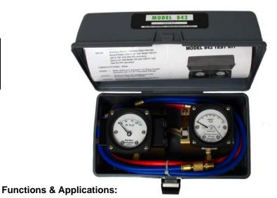
Rugged (2) gauge medium duty portable flow test kit. This kit is equipped with two differential pressure gauges (1) Diaphragm Type and (1) Piston Type gauge with complimentary dials ranges. Both gauges are protected against over-range to the maximum working pressure of the test kit. While primarily used for balancing HVAC systems it has numerous other applications which include but are not limited to: checking pump performance, checking pressure drop across filters, leakage, etc...
