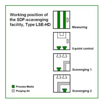
The function of the purging facility is to clean both chambers of the connected sensor with compressed air in order to avoid respectively remove clogging of and from the bore-holes. First of all the flanged-on differential pressure transmitter has to be disconnected at both ends from the pressure piping. Then both pressure pipes including the sensor chambers will be put under compressed air and purged separately and one after the other. Central element of the
