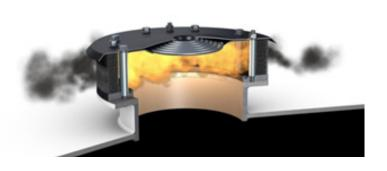
of explosion pressure in the process equipment the flame arrester is used to dissipate the energy of the expelled combustion flames into its material. By reducing the gas temperature to a safe level, flameless venting can be used in areas where it would be impossible to safely use an explosion vent only.
