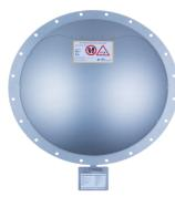
Filter installations with pneumatic cleaning systems and a very high vacuum operation require an explosion vent that withstands vacuum and positive pressure cycling for a long time. For such requirements the GE is the best choice. Its domed design enables negative pressure resistance without the need for an extra vacuum support. The GE type vents feature pressure peak damping as well as integrated flange gaskets.
