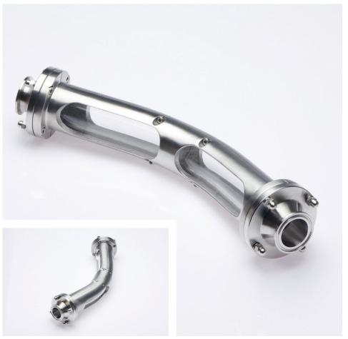
The **Curved SVFI** has been developed to overcome issues inherent in the processing industry. As it can be difficult to view the middle of a bend without equipment such as boroscopes, it is not easy to ensure the cleanliness of a system. Surface finish cannot be guaranteed at the middle of a bend as it is inaccessible to measuring equipment and not all bends are 'piggable', due to their manufacturing method.
